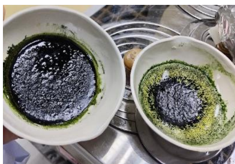
Figure 1: The evaporation process of extracting solvents by using hot plate and the final product of Carica papaya leaf extract.
